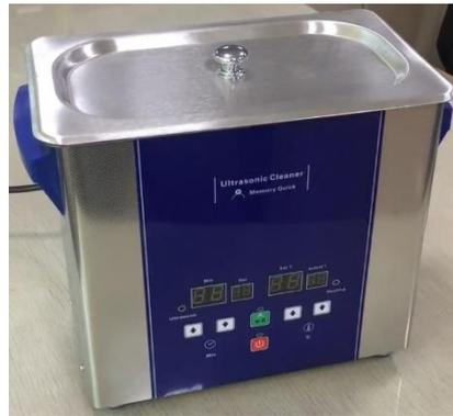
**Figure 4:** *Sonication for mixing nano particles.*
